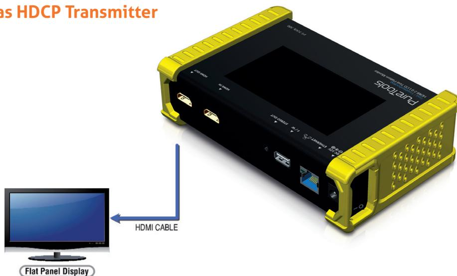
When PRO-HDMI2Gen set as transmitter, it can transmit HDCP encrypted video. PRO-HDMI2Gen also provides three modes (HDCP 1.4 / HDCP 2.2 / no HDCP) for you to select. If user wants to transmit HDCP encrypted video again, please select the Auto-Restart button.
