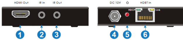
Figure 3: HDBaseT Receiver Layout
