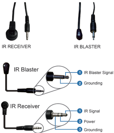
Figure 5: IR Cable Pin Definition
